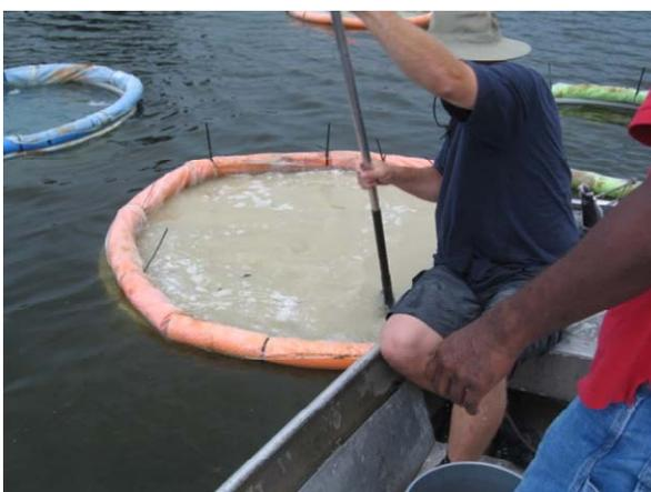
Slurry mixed into chamber with paddle
