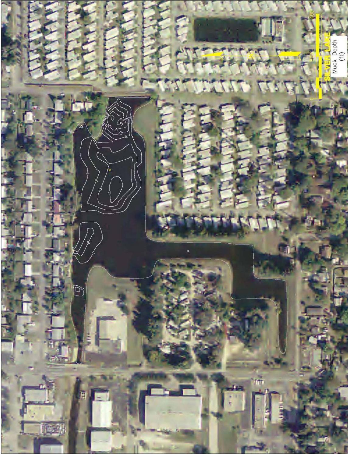
Figure 2-3. Depth Contours of Unconsolidated Organic Sediments in Silver Lake.
