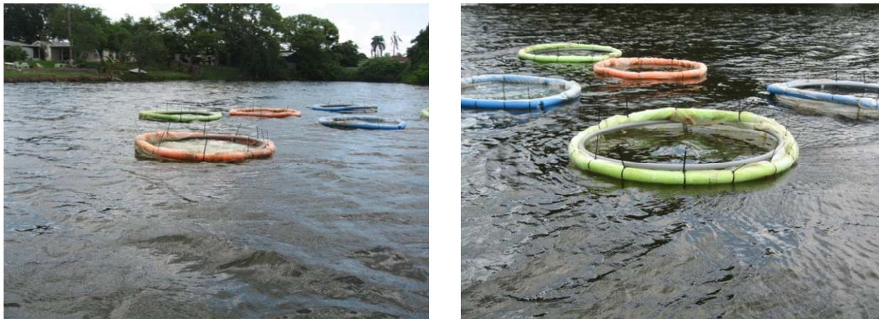
Figure 3-6. Completed Limno-Corrals with Floating Isolation Bags.
