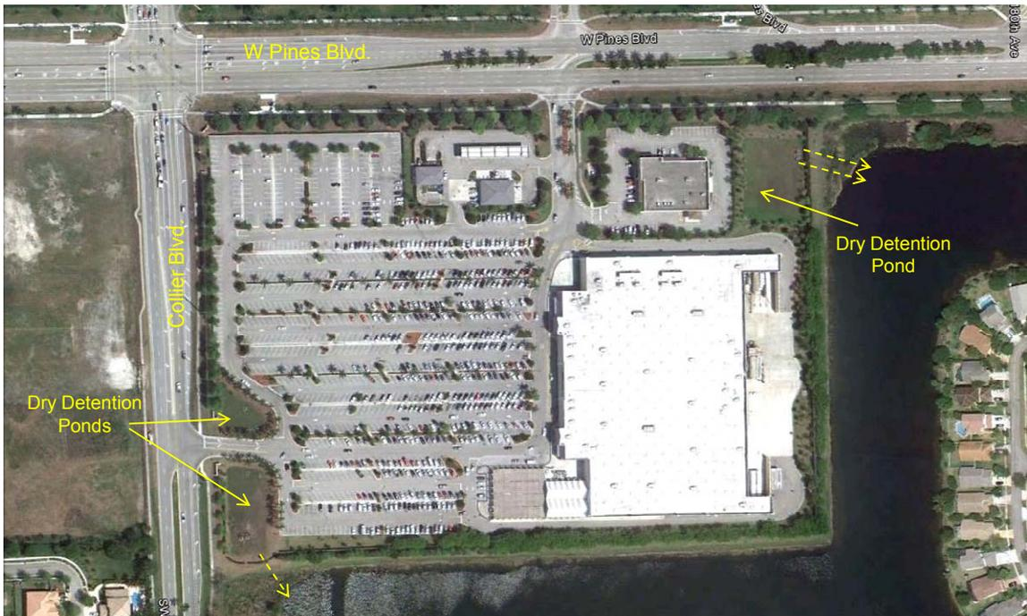
Figure 2-16. Overview of the Pembroke Pines Dry Detention Site.
