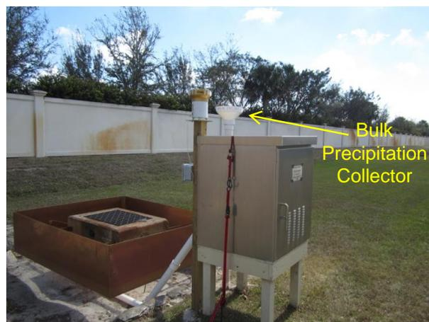
Bulk Precipitation Collector at Naples
