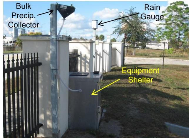
Site 4 – Equipment Shelter, Rain Gauge, and Bulk Precipitation Collector
