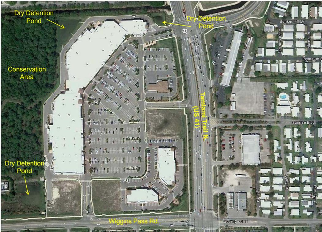
Figure 2-6. Overview of the Bonita Springs Dry Detention Site.
