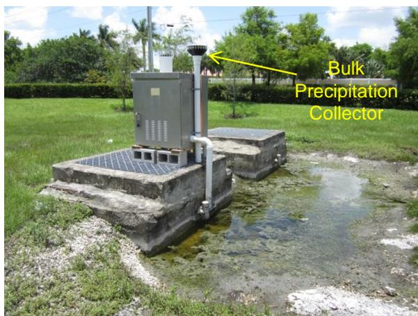
Bulk Precipitation Collector at Pembroke Pines
