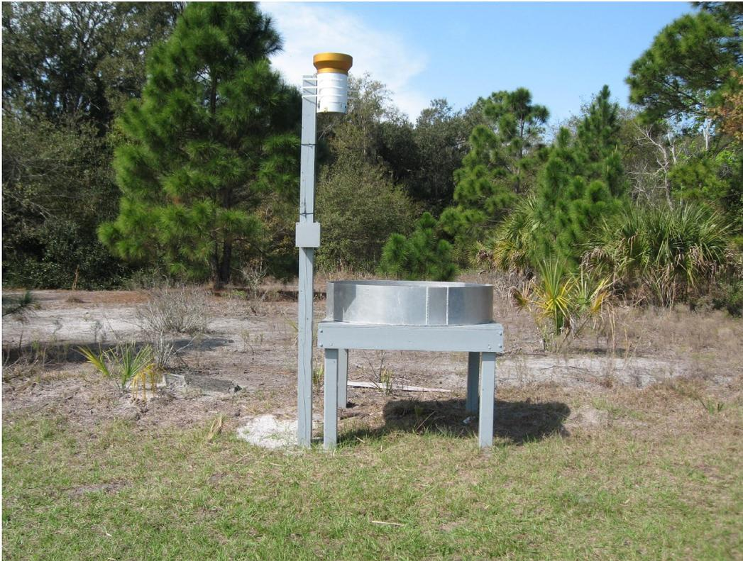
Figure 2-4. Rainfall and Pan Evaporation Equipment.
