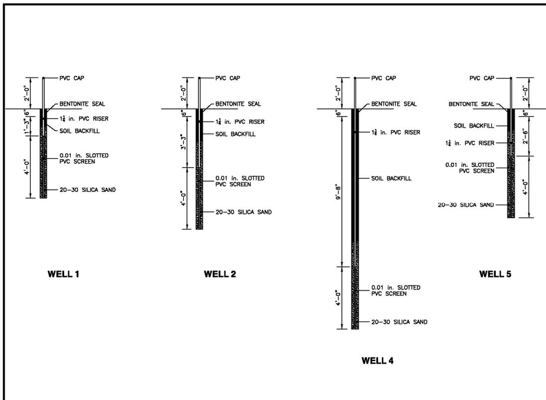
Figure 3-20. Construction Log for the Shallow Monitoring Wells.
