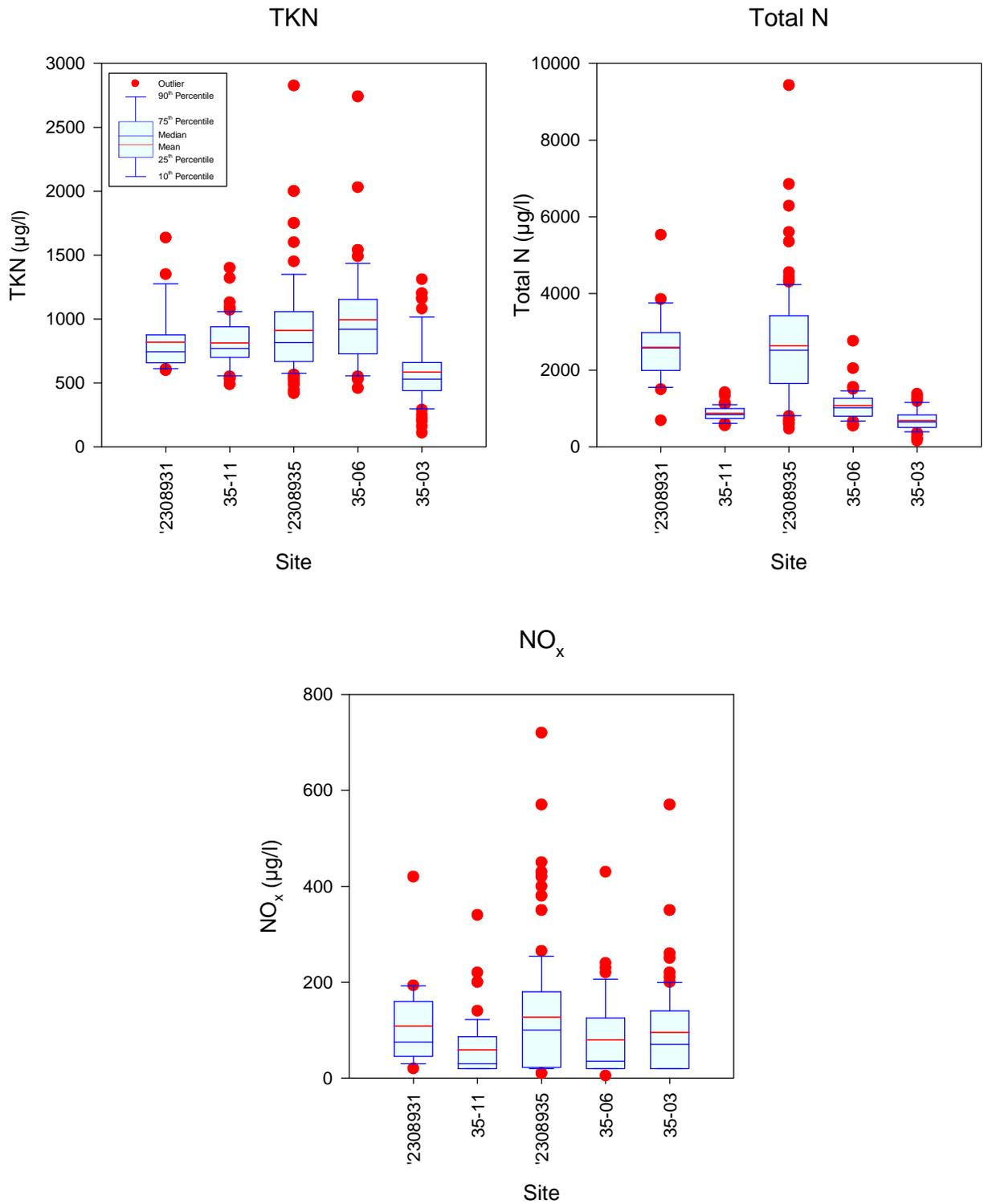
Figure 2-26. Statistical Comparison of Historical Water Quality Data for Nitrogen Species in the Freshwater Segment of Joe’s Creek.
