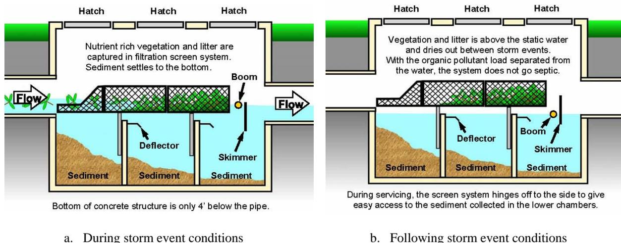
Figure 2-4. Schematic of the Suntree 2<sup>nd</sup> Generation Nutrient Separating Baffle Box.
