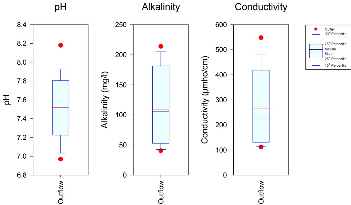
Figure 4-44. Statistical Summary of Outflow Concentrations of pH, Alkalinity, and Conductivity at the Lake Concord Suntree Baffle Box Site.
