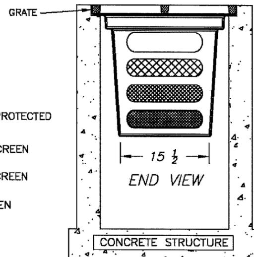
REMOVE GRATE INSERT GISB REINSTALL GRATE
