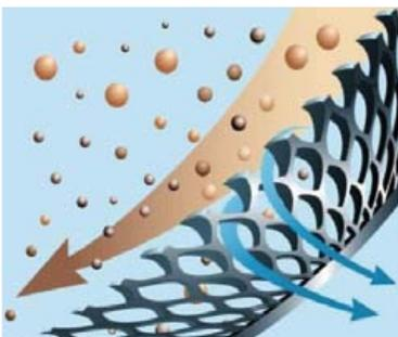
Continuous deflective separation — water velocities within the swirl chamber continually shear debris off the screen to keep it clean
