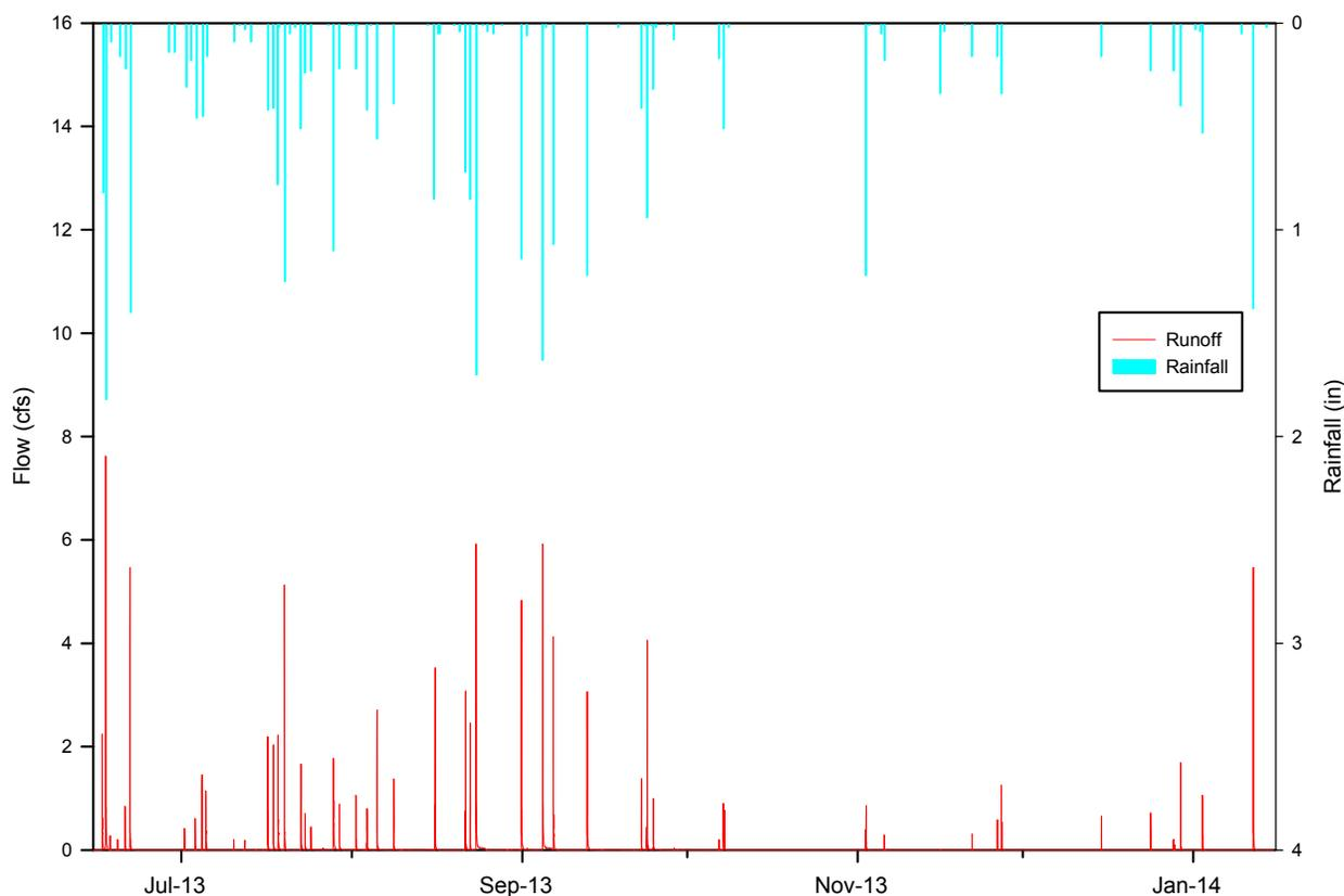
Figure 4-6. Measured Runoff Hydrographs at the Lake Concord Suntree Baffle Box Site from June 15, 2013-January 15, 2014.
