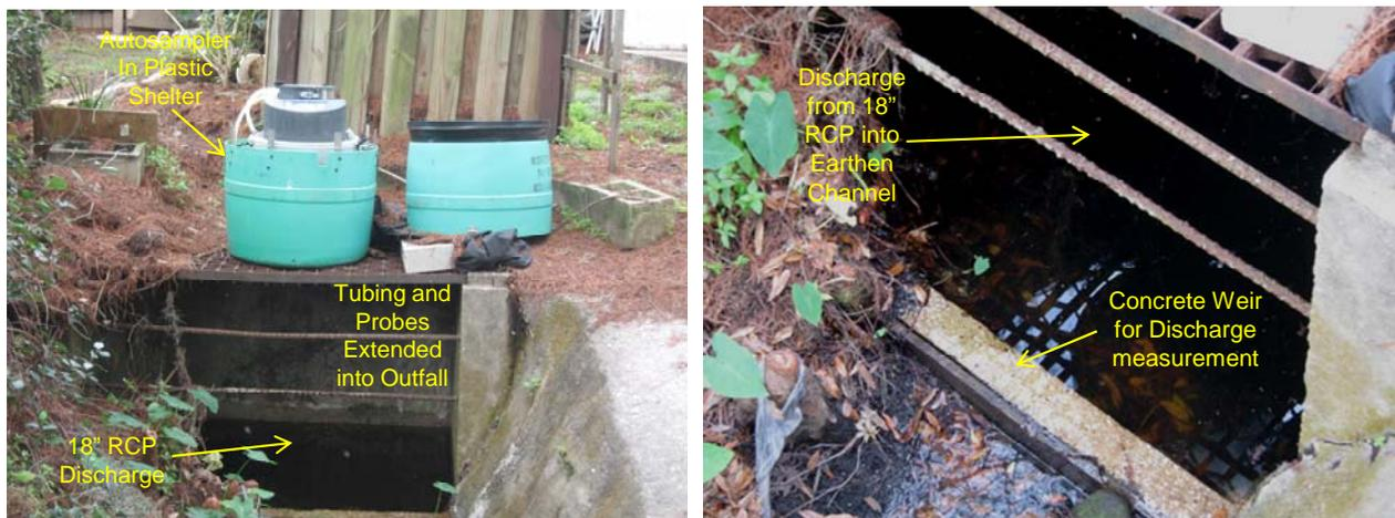
Figure 3-6. Photographs of the Sampling Equipment Used at the San Pablo CDS Unit Site.
