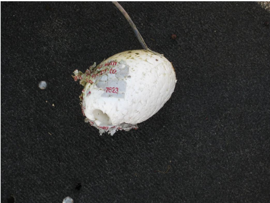
Figure 2-4. Example of Bite Marks on Seepage Meter Floats.
