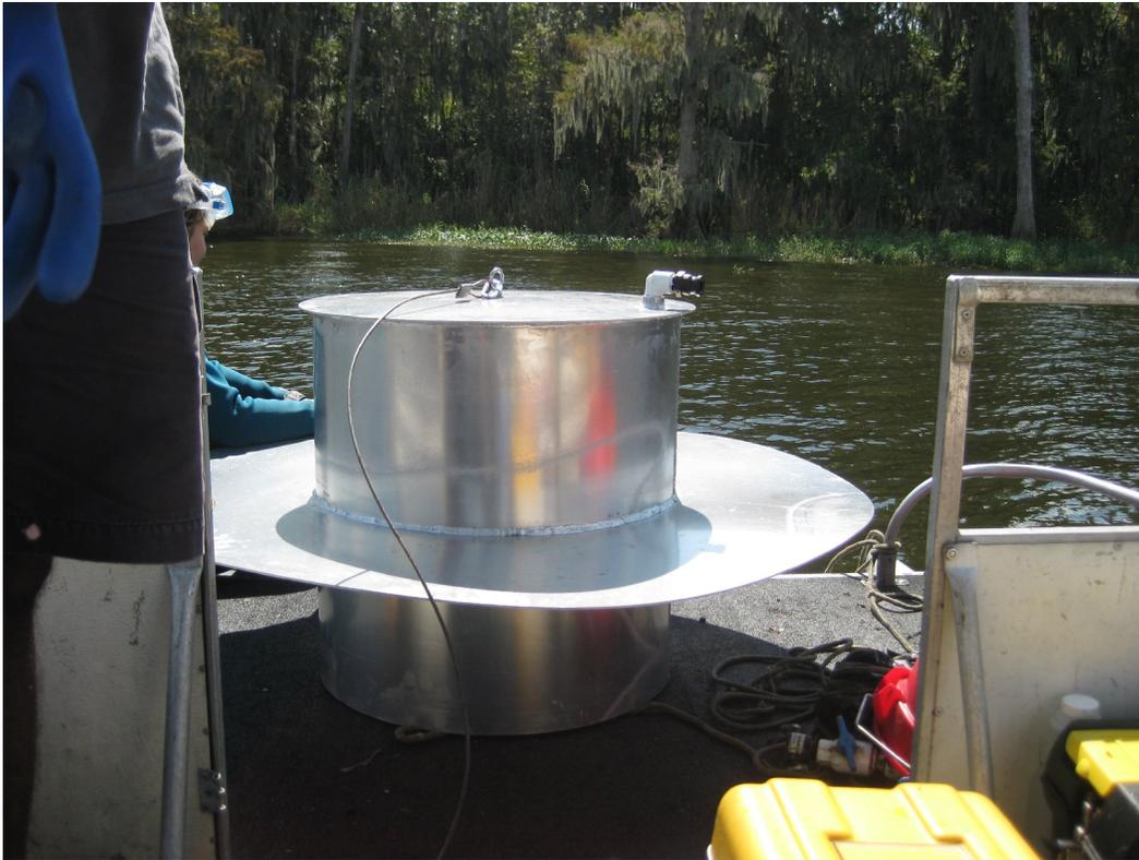
Figure 2-2. Typical Seepage Meter Used in Lake Jesup.
