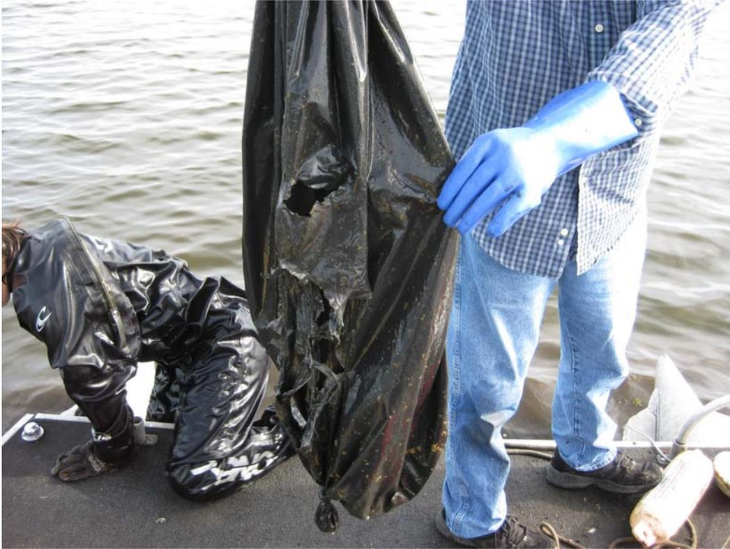
Figure 3-2. Example of Damaged Seepage Collection Bag.
