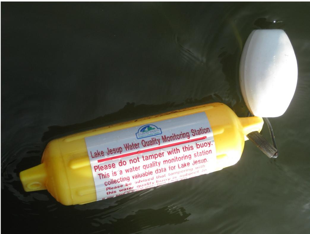
Figure 2-3. Floating Buoy Used to Identify Seepage Monitoring Sites.
